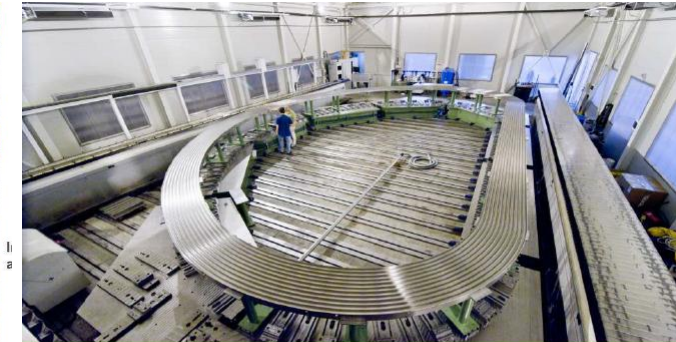
The radial plates that hold the conductor of the toroidal field coil: D-shaped stainless steel structures with grooves machined on both sides along a spiral trajectory.
